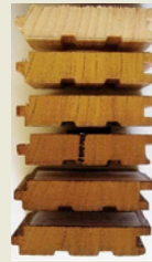
Colour darkens as the temperature in the process is increased
